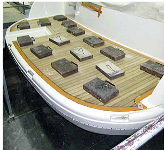
Fig. 27 Holding in place with weights
