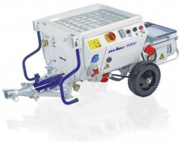
Roto-stator worm compact pump, e.g. MTEC P20 400 V. With a maximum pressure of 30 bar and maximum 30 m of hose. It may require an external mixer. For small repairs, e.g. 1 manhole ( \varnothing < 1 m)
