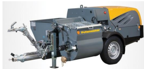
Roto-stator worm pump, e.g. Putzmeister P11 SP 16.2 KW. With a maximum pressure of 30 bar and maximum 52 m ( \varnothing 50 mm) of hose. No external mixer required For large repairs
