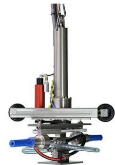
Spin Casting Machine. For manholes where no bends or irregular shaped portions are found. Only for repair of manholes
