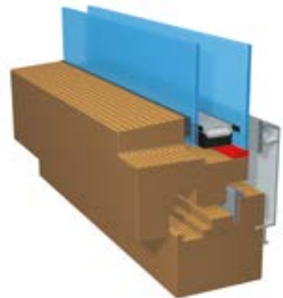
Glass Edge Bonding with Sikasil® WT Technology
