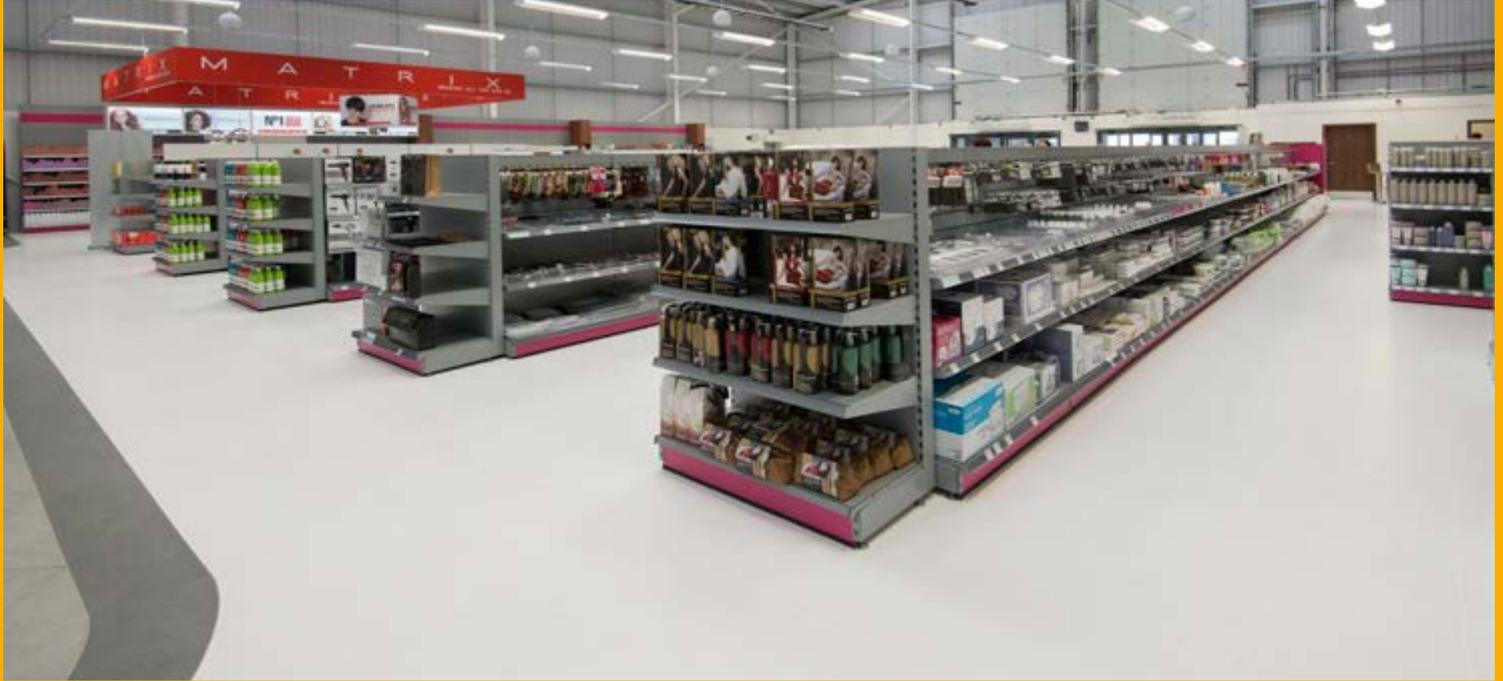
[Sikafloor®-161](#) also provided an integral Damp Proof Membrane (DPM) to prevent moisture from passing into the open interior warehouse space.
