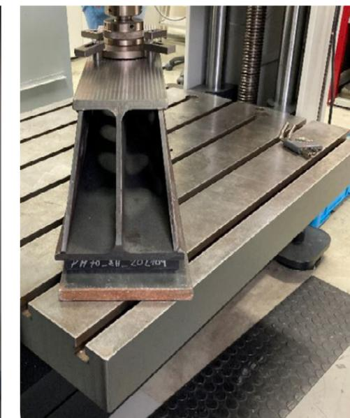
Discrete/Direct fixation test.
