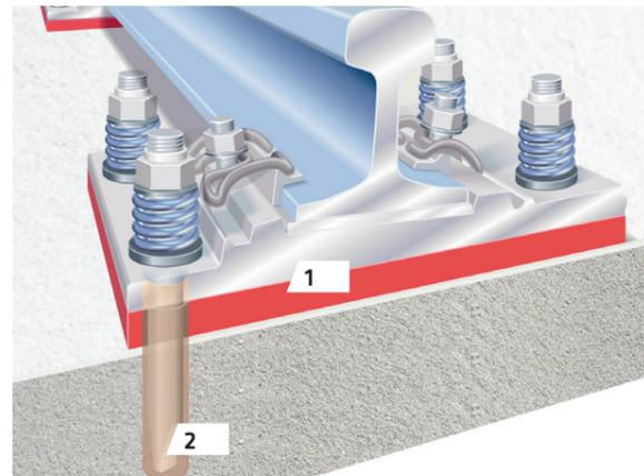
On the discrete fixation of rails the single fixations will be fixed by anchor bolts and stored on Sika® Icosit® KC.
