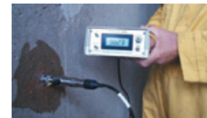
Permeability Testing of Concrete
