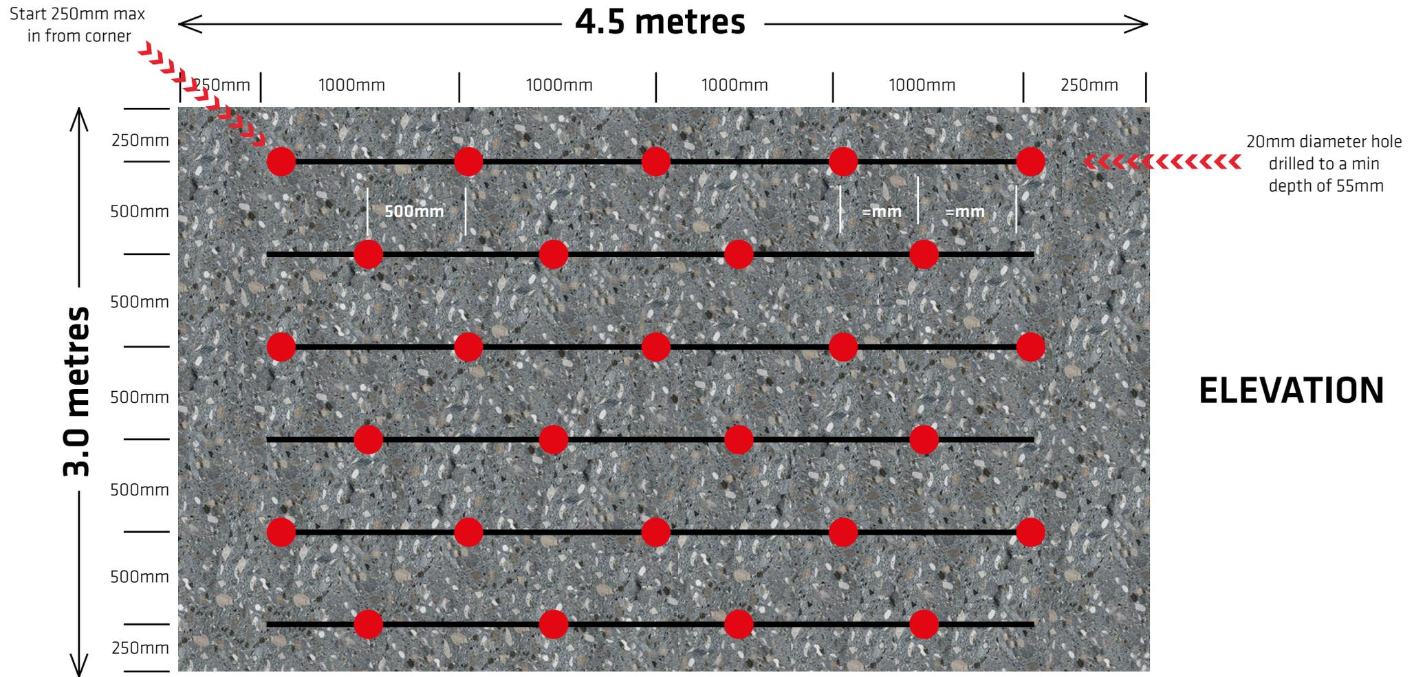
The above example is a recommendation of cartridge placement for a wall of 4.5metres by 3.0 metres. The important factor is to ensure even spacing through out and minimum dosage rate of 2 capsules per m<sup>2</sup> of surface area. For concrete depth over 500mm where corrosion protection is required, it is recommended to increase the dosage rate to 2 capsules per hole and staggering the insertion depth.
