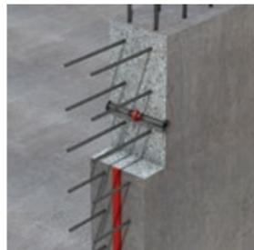
X-Plugs and SikaSwell® Rings are an easy and secure way of sealing around all types of formwork spacers. Different sizes are available for most common spacers. The SikaSwell® Ring seals around the outside of the spacer while the X-Plug seals the inner side.
