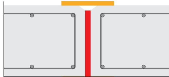
Where internal waterstops are used, correct fixing is essential to keep the waterstops in place during the concreting operations. Good compaction of the concrete around the waterstops is also necessary to avoid paths for water ingress.
