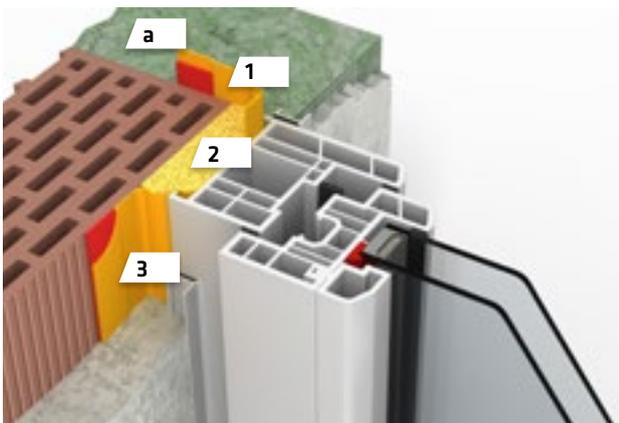
**1** SikaMembran® Window Outside bonded with SikaHyflex®-220 Window
