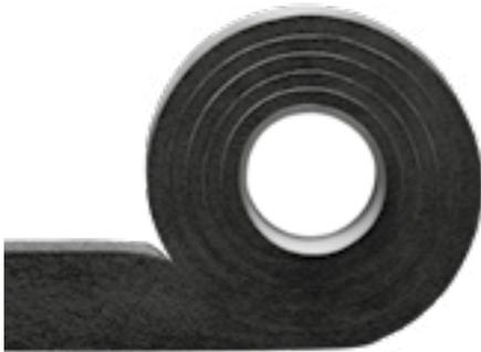
Expansion tape used for thermal insulation between frame and adjacent construction. To seal against driving rain, sealants are required in addition (use SikaHyflex®-220 Window).
