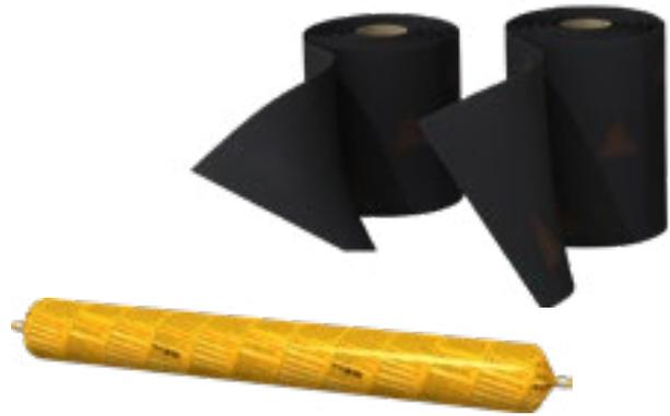
The high quality system consists of indoor and outdoor membranes, which are bonded with Sikaflex® TF Plus N to the façade element and the building construction. This system is especially suitable for curtain wall facades, wide connections and multi-storey buildings with high demands through wind forces and UV radiation.
