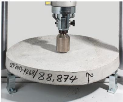
Round panel test: ASTM C1550
