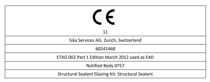
The assessment of the fitness for use of the structural sealants for the intended use in relation to the basic requirements for construction works are carried out in accordance with ETAG 002 - Part 1.
