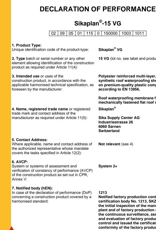
15 VG (lot no. see label and product) Polyester reinforced multi-layer, synthetic roof waterproofing sheet based on premium-quality plastic compound
