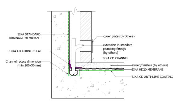
The membrane is rolled out 'studs down' over the floor, and consecutive sheets are laid so the flanged edge overlaps the first sheet by four studs. Joints are sealed using Sika® Jointing Tape applied between the second and third row of studs. Joints without the flanged edge are overlapped by four rows of studs and sealed with Sika® CD Rope applied between the last two rows or over sealed using Sika® CD Overseal Tape.
