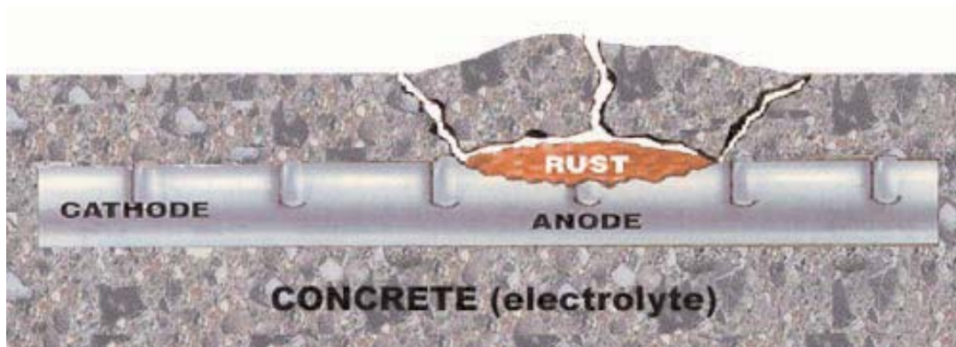
Figure 2: Formation of rust causing spalling of concrete
