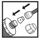
**2.** Fit the cartridge outlet plug into the cartridge then place injection resin mixer nozzle onto the cartridge.
