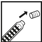
**5.** After bonding on the injection ports, remove the tip from the static mixing nozzle.
