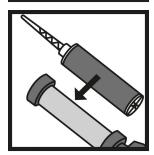
**4.** Place the cartridge into the application gun ready for use. Pump gun until both resin parts are extruded as one mixed consistent colour. Do not use unmixed material.
