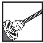
**3.** Slide the screwcap over the injection resin mixer nozzle and screw onto the cartridge.
