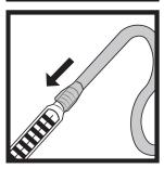
**5.** Fit the flexible extension hose onto the injection resin mixer nozzle.
