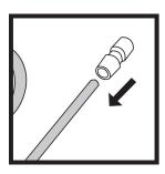
**6.** Fit push fit connector onto the hose. Pump gun until both resin parts are extruded as one mixed consistent colour. Do not use unmixed material. Place connector over an injection port and start the injection application.
