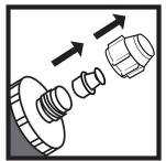
**1.** Unscrew the screwcap (do not throw away) and remove the plug from the cartridge outlet.
