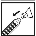
**6.** Fit the applicator fan onto the square mixing nozzle then start the crack sealing application.
