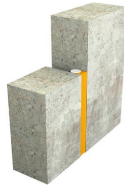
PE backer rod and fire resistant sealant
