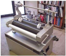
Follow the guidelines below or the Manufacturer's procedures for proper machine set-up and calibration. Rollers are calibrated to saturate the fabric with the correct resin-to-fabric ratio. Have the pre-cut fabric ready or a roll of fabric positioned on the saturator. Use the saturator according to the manufacturer's manual.
