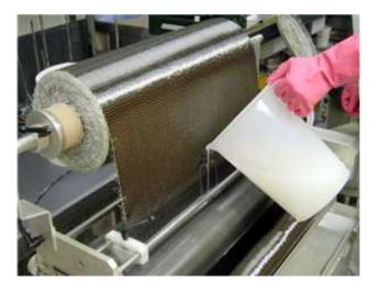
Continuously pour resin onto the rollers on both sides of the fabric
