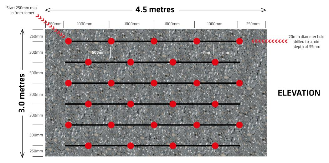
The above example is a recommendation of cartridge placement for a wall of 4.5metres by 3.0 metres. The important factor is to ensure even spacing through out and minimum dosage rate of 2 capsules per m² of surface area. For concrete depth over 500mm where corrosion protection is required, it is recommended to increase the dosage rate to 2 capsules per hole and staggering the insertion depth.
