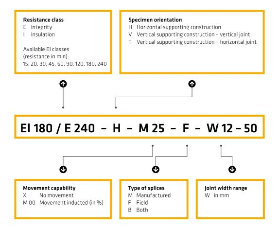
You may be asked the question: "Is your fire resistant joint seal able to accommodate movement?" Be careful! – It is not enough to use an elastic joint sealant with the required movement capability (e.g. according to ISO 11600 or ASTM C 920); because specific fire resistance tests (e.g. according to EN 1366-4) must also be performed under forced movement.
