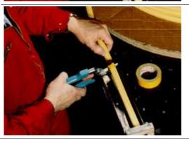
Cut the PVC installation and vent end hoses, green and transparent, to the desired lengths. Apply superglue to the connecting nozzles to ensure a secure connection.
