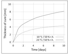
Diagram 1: Curing speed for Sikaflex®-552
