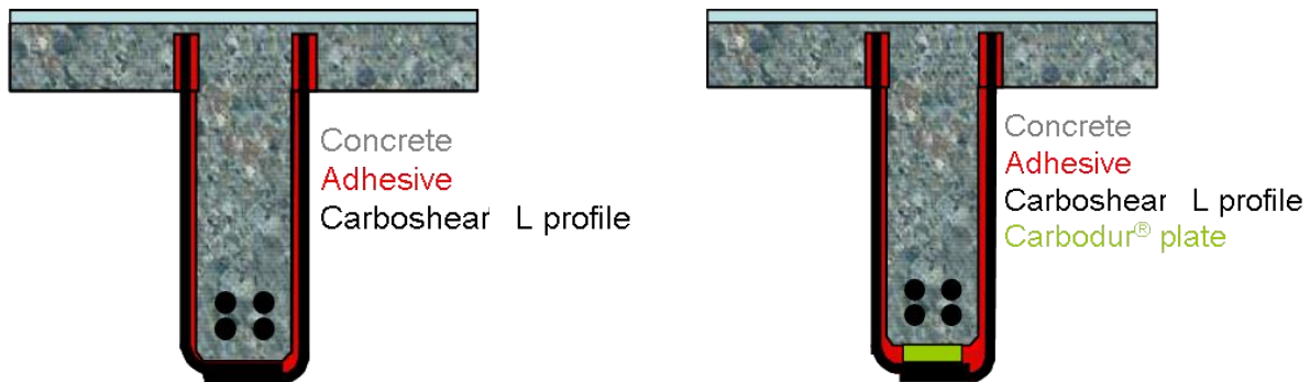
Sika® CarboShear for shear strengthening and improved end anchorage of Sika® CarboDur® Plates
