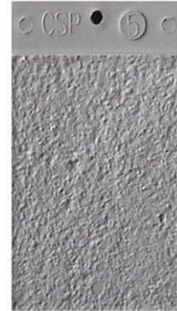
CSP-5: Medium Shot Blast / Bush-hammering
