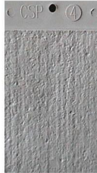
CSP-4: Light/medium shotblast light scarification/ Bush-hammering
