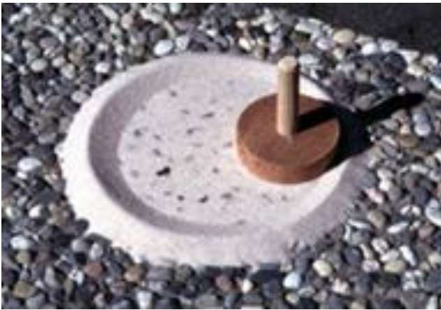
A defined sand quantity (volume V ) has to be distributed onto the surface in a circular manner so that all deepenings are filled exactly with quartz sand.
