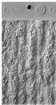
CSP-9: Heavy Scarification
