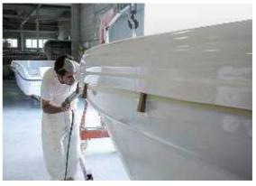
For satisfactory results the adhesive must be applied with adequate equipment such as a piston application gun. Sikaflex®-591 can be overpainted with most conventional marine paint systems.
