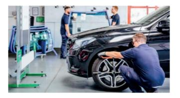
Therefore, after the replacement and prior the vehicle being handed over to the driver, a recalibration of ADAS is needed to secure road safety. Independent of the climate or the location that the replacement of the windshield is executed. The installation and calibration must be precise and follow a defined process.
