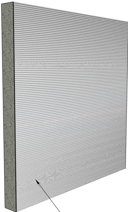
• SIKAPROOF ADHESIVE 02 Applied by 4 mm notched trowel. Adhesive is then smoothed before applying SIKAPROOF A+ MEMBRANE
