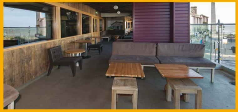
To create the hard-wearing floor, a three component Sikafloor<sup>®</sup> Pronto system – comprising primer, levelling mortar and a fast curing top coat - was applied within just 5 working days. In addition to exceptional waterproofing abilities, the self-smoothing screed and levelling mortar was scattered with quartz sand to resemble a sandy beach whilst maintaining the watertight and slip resistant surface.
