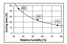
$<sup>^{5)}</sup>$  Curing time for 500  $\mu m$  adhesive film at 20  $^{\circ}C$
