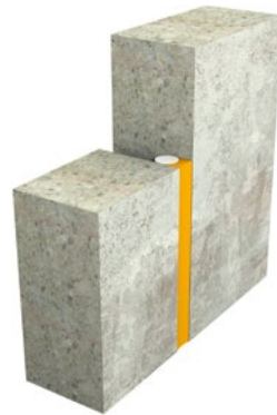
PE backer rod and fire resistant sealant
