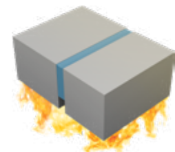
8/9. Single seal, exposed or unexposed side
