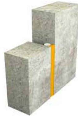
PE backer rod and fire resistant sealant
