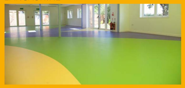
Consisting of a soft polyurethane resin combined with a rubber crumb matting which gives added cushioning underfoot, <u>Sika® ComfortFloor®</u> <u>Pro</u> from Sika proved ideal for the children and staff at Rainbow House. The system's chemical composition and texture absorbs impact and offers the perfect surface for intensive therapy work taking place at the facility, while also providing a high degree of comfort for the children.
