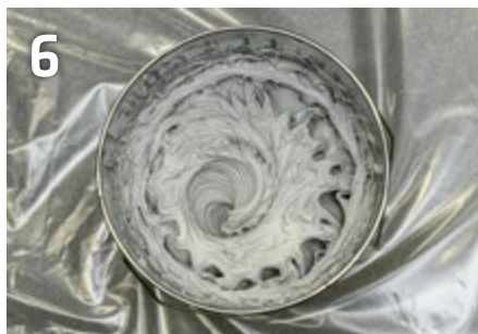
6 Ensure that both materials are completely blended, including on the container edge and on the bottom.
