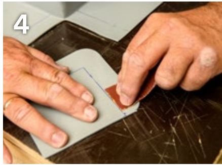
4 Roughen the overlap and/or weld with sandpaper.
