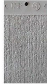
CSP-4: Light/medium shotblast light scarification/ Bush- hammering
