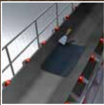
Conveyor belt repair and bonding
