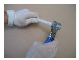
3. Remove the retaining nut
