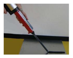
9. To ensure uniform thickness of adhesive when compressed, we recommend to apply the adhesive in the form of a triangular bead.
