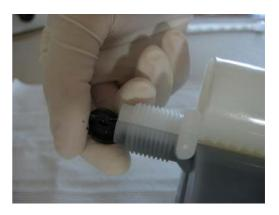
5. Put the static mixer on the cartridge with the retaining nut
