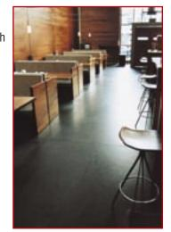
surface hardening system in a classic grey colour. As well as satisfying all requirements, being integral with the floor slab this system was much faster than overlaying with conventional floor coverings.
