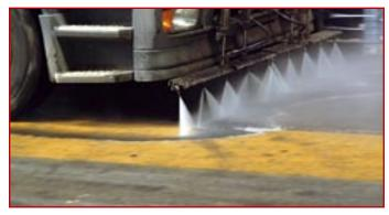
**Sikafloor®-20 PurCem** also had to cope with the high residual moisture in the slab resulting from the daily washdown of the road sweepers. The whole job was completed within a 27 hour time window by Mitie Flooring.
