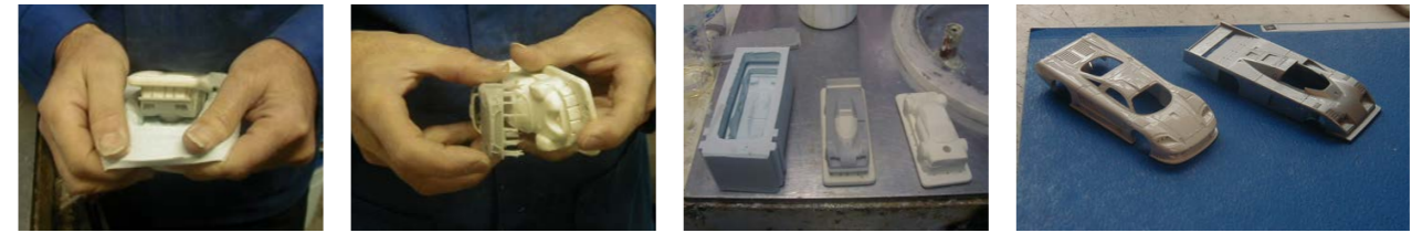
SikaBiresin® F38 is ideal system to produce small figurines with sharp details and excellent resistance in thin layers
