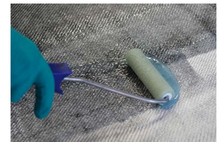
Wet lay-up with SikaBiresin CR168
