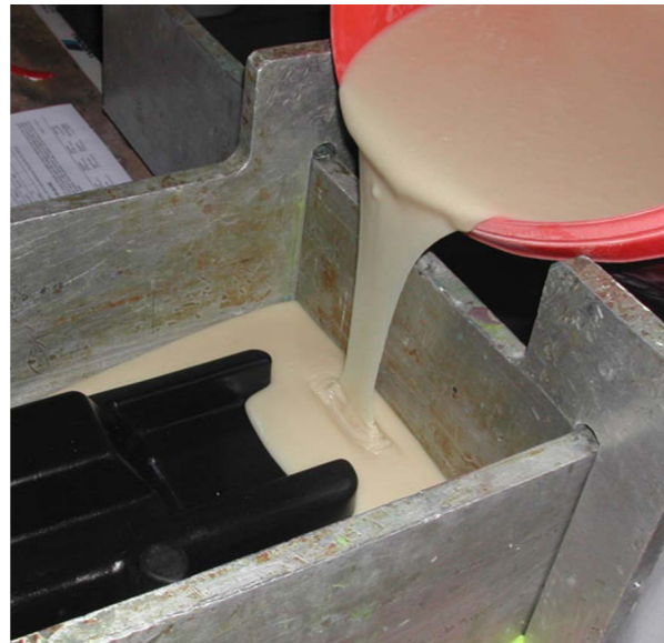
SikaBiresin® F46 ready-to-use and both refillable F48 or F50, are slow systems allowing manual casting of very large size negatives, patterns or moulds with minimal shrinkage
