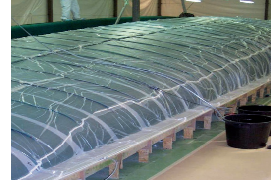
Vacuuminfusion with SikaBiresin® CR131
