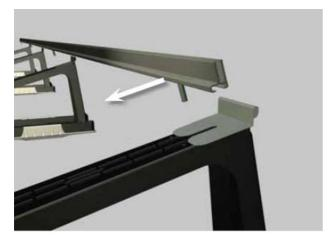
Place the second rail with pre-mounted hammer-head screw in the slots provided.
