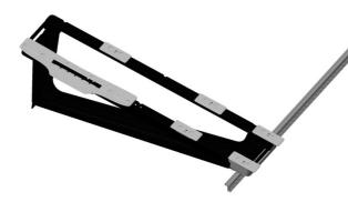
Prepare an assembly rail with the pre-assembled screws. Turn the mounts with the Sika SolarClick, base plates and the UV cap upside-down and insert the hammerhead screws in the provided mounting aperture at the lower end of the mount (South).
