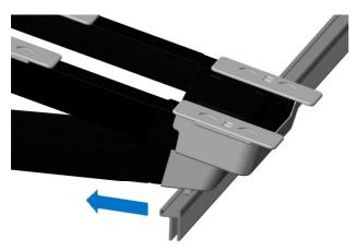
The ridge of the module assembly rail must be facing the centre of the mount
