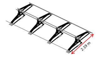
Position the opposite frame (same construction and distances) at the rear side of the first frame. Overlap of the mounts is 0.20 m.
