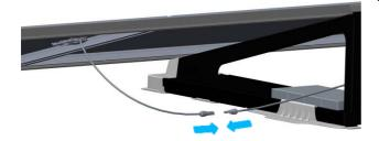
Interconnect the plugs while joining the modules.
