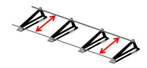
Insert assembling jigs with the width of a module (see red arrows let) on both sides between the mounting rails in order to establish the exact distance to one another, and then remove the jigs.
