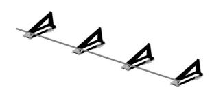
Once all mounting racks are firmly connected to the assembly rail, these are placed back on foot by turning them by 180°.
