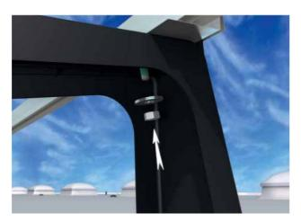
Fix the washer and the nut to the hammer-head screw.
