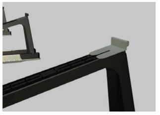
Stick the wind deflector cap onto the mount nose. In case of the East-West system they serve as protection against UV radiation.
