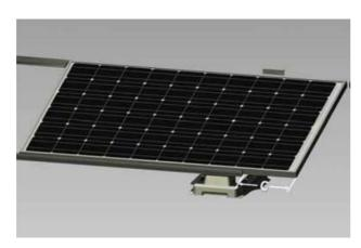
Lay the first module onto the bases of the module assembly rails and set up the module cantilever (c) according to the previous table or the layout plan.
