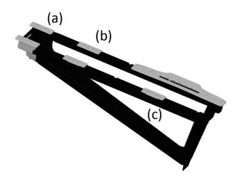
5 additional base plates are mounted to the underside of the mount:
