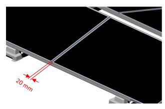
Insert the remaining modules with a distance of 20 mm to the adjacent modules. The junction boxes of the modules should face to the same side.
