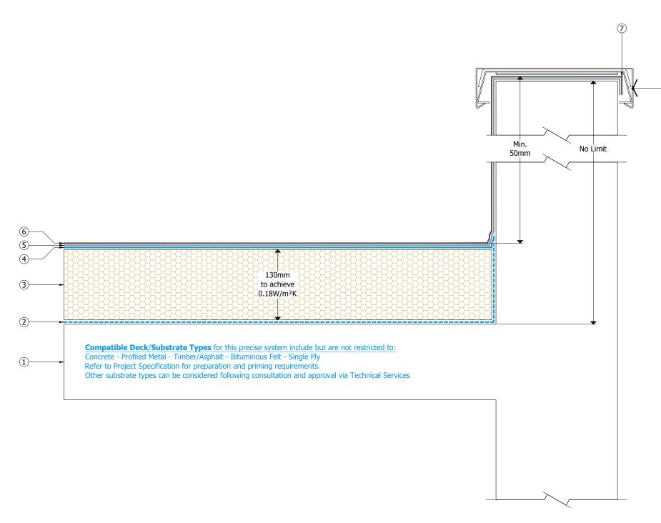
New or existing reinstated metal cappings; all mechanical fixings used in the capping system must be encapsulated to prevent water ingress
