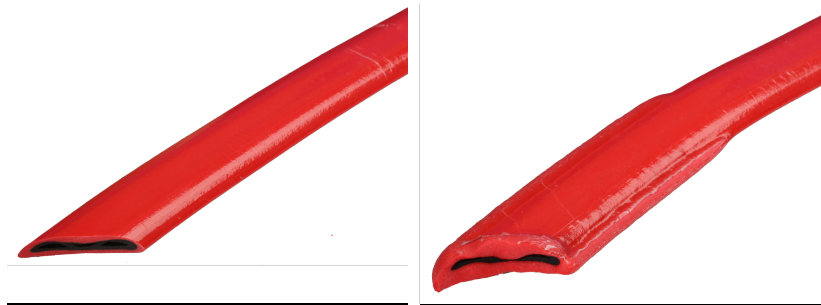
Profile before swelling (left) and after swelling (right)
