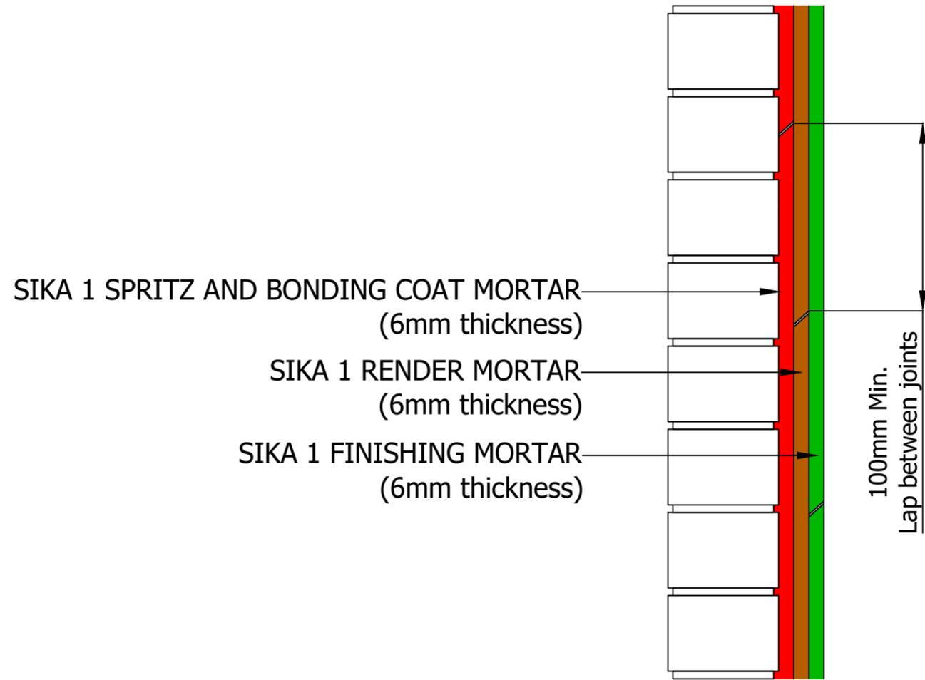
SIKA 1 SPRITZ AND BONDING COAT MORTAR
