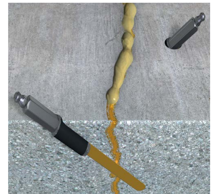
Figure 10. Digital image showing a sectional view of high pressure crack injection
