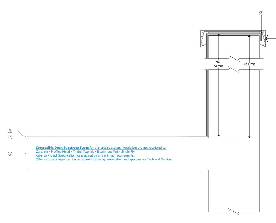
New or existing reinstated metal cappings; all mechanical fixings used in the capping system must be encapsulated to prevent water ingress
