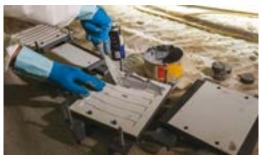
Pull-off test to test cohesive strength of concrete substrate after surface preparation  $\uparrow$
